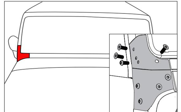
4. Install assembly to vehicle using supplied 5/16" button head bolts and washers. Adjust fitment if necessary and securely tighten all bolts.
