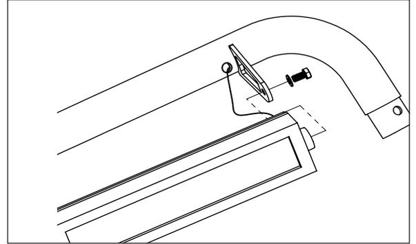
2. Attach LH and RH brackets to crossbar with supplied M10 button head bolts, M10 Flat Washers, and M10 lock nut. Do not tighten completely to allow for adjustment.
